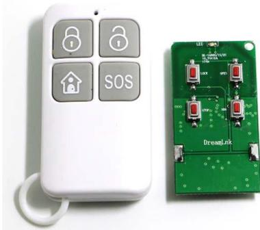
Figure 3: Module connect to buttons
