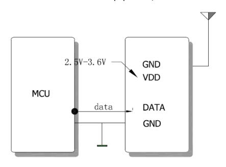
Figure 2: Wiring diagram for module application
