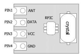
The DL-TXS868T module has 4 pins, which are defined in the following table
