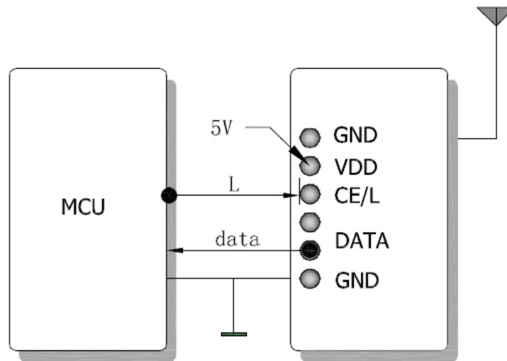
Figure 2: Wiring diagram for module application
