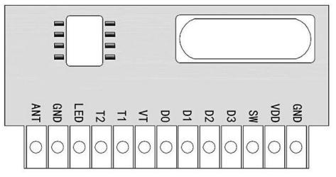
Figure 5 DL-RXC6B Module interface definition diagram
