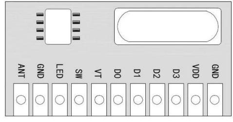
Figure4 DL-RXC6A Module interface definition diagram
