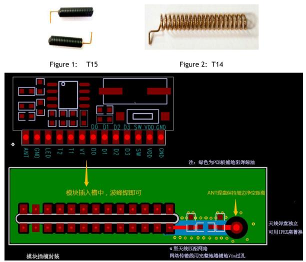
Figure 3: Schematic diagram of module insertion and antenna layout
