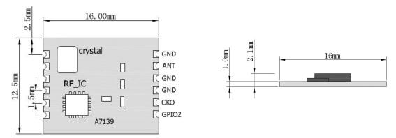
Remark: Gold plating PCB with half hole stamp edge and surface mounting technology (SMT) as defaulted. To avoid the resistance damage of high-power iron during mass production, please do not weld the antenna directly to the module.
