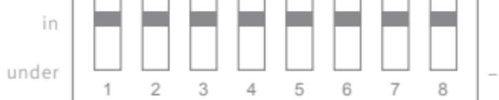
2. Find the code table on the back of the original remote control: Switch the dial switch according to the code table, make the 8 switches same position as the original remote control, the new remote control can be used when the code is consistent.
